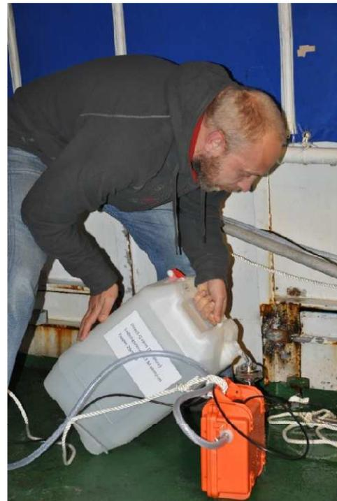
Figure 3 Control sampling, 25 liter MilliQ
